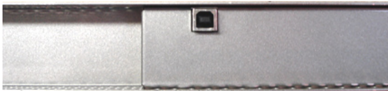
Fig. 4 - Section of back of bezel with USB B-type plug
